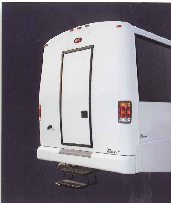
▼ The Classic Coach's rear cap provides distinction with no exposed hinges.
