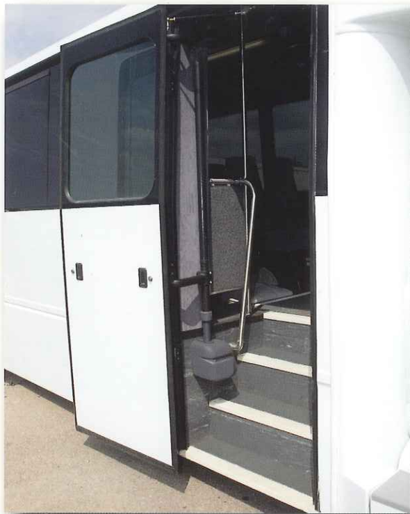
▲ Plug-style entry door provides room for easy passenger entry.
