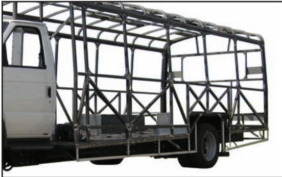
1 1/2" x 1 1/2" Steelguard® construction provides superior durability.
